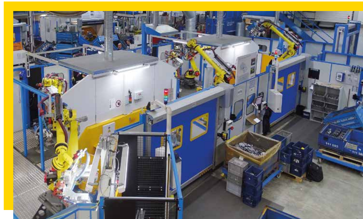
One of the new welding lines for the VW MEB platform at the Attendorn plant.
