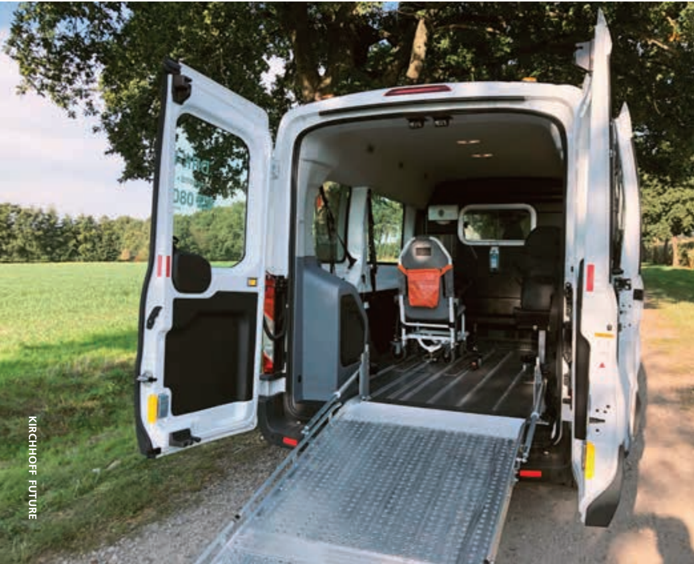
The carrying chair allows patients to be transported in a sitting position. This facilitates the daily work of the DRK team.
