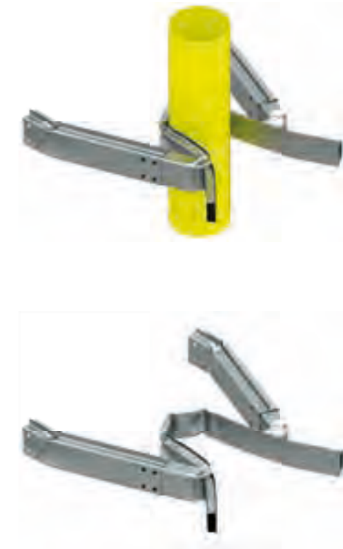
Advanced crash management system with high deformation capacity.
