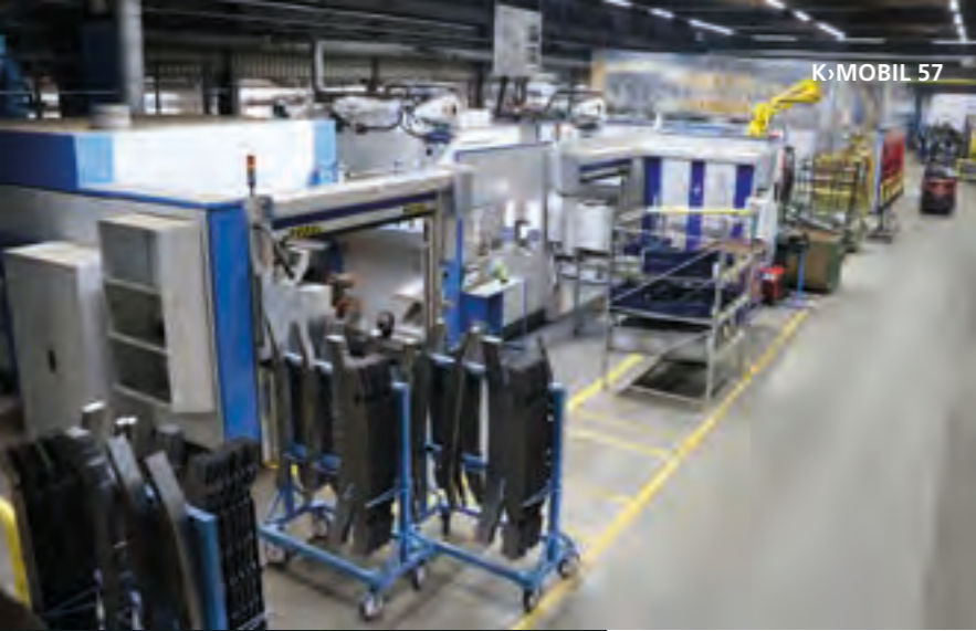
top: New production line with fully automated process steps module 1: laser welding module 2: handling and fastener welding module 3: MAG welding and inline rework module 4: handling and discharge of the finished cross-member assembly bottom: Seam tracking sensor for exact positioning of the laser beam.
