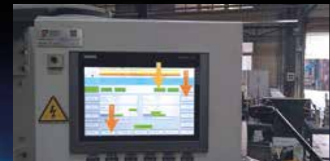
Online view of the specialist on the user's environment. The specialist can insert visual cues, which are projected directly into the user's field of view by means of the glasses.
