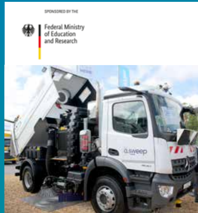
FAUN presents a.sweep, the concept of an automated driving sweeper. This project has emerged from the Transatlantic Autonomous Driving Alliance (TADA), whose aim is to create a network linking US and German companies around new vehicle technologies. The project is funded by the German Federal Ministry of Education and Research (BMBF) and the Michigan Economic Development Corporation (MEDC).
