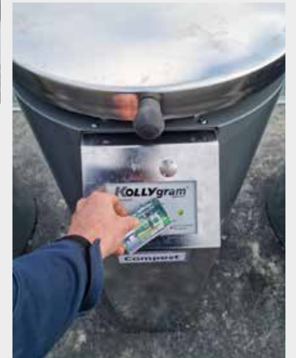
Identification of the customer takes place via a card reader
