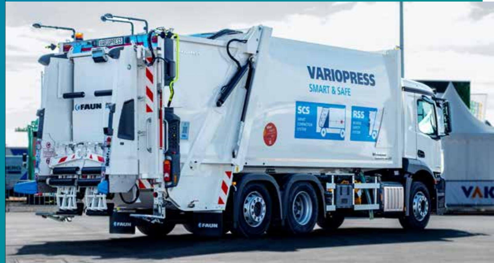
Smarter and safer refuse collection vehicle: VARIOPRESS with Smart Compaction System (SCS) for the automated and energetic optimized control of the compaction in the refuse collection vehicle and the Reversing Safety System (RSS) to prevent accidents in the rear area of the refuse collection vehicles.
