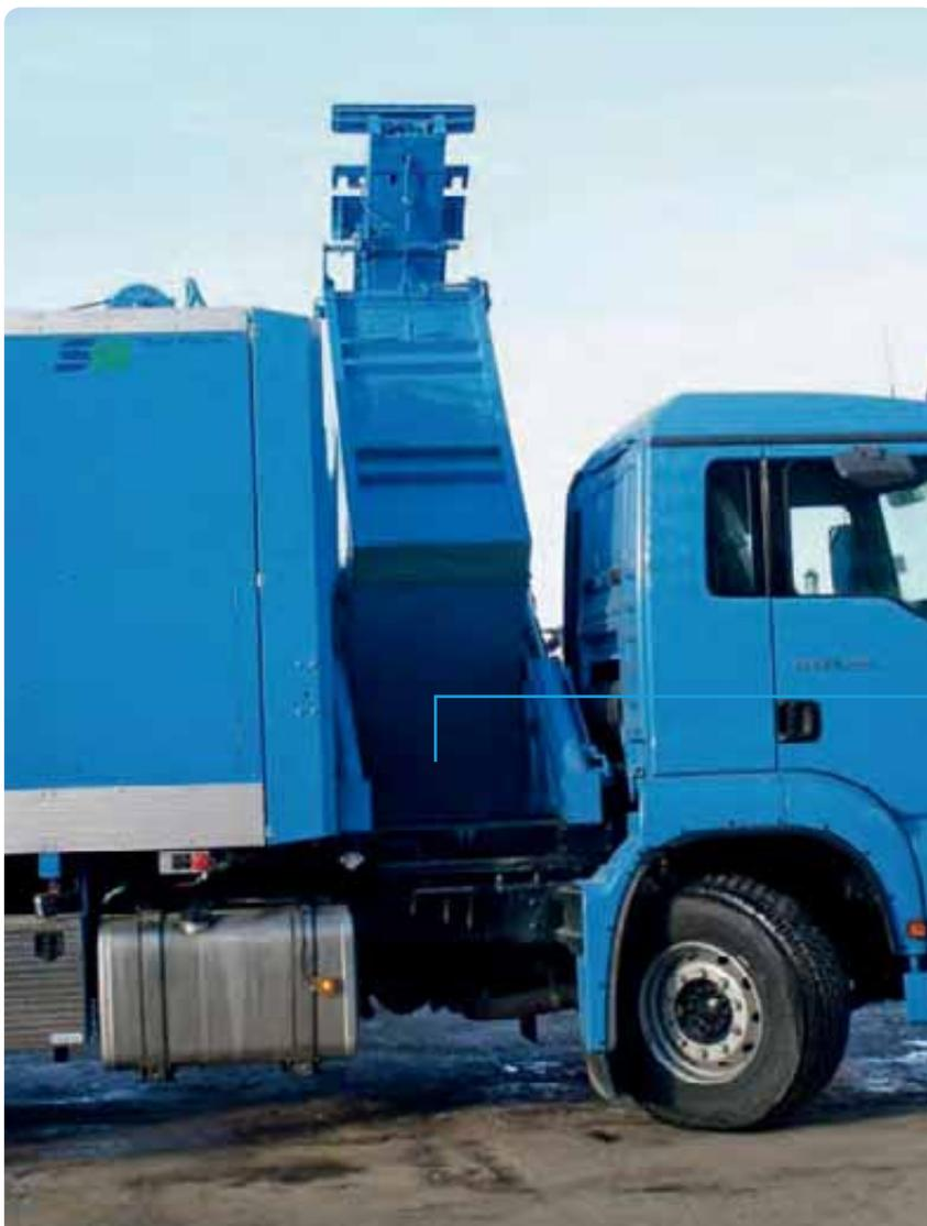
*Bio or glass box in tipping position, for lateral emptying. The bio box is also available in a stainless steel version.*
