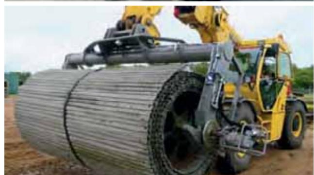
**Left:** MGMS-BD prevents vehicles from getting bogged down. **Right top:** MGMS-BD LITE, a lighter, cost-effective option. **Right down:** A standout feature of the MGMS-BD is its rotating head, allowing the system to be rotated 180 degrees so the plant can fit through smaller gaps, further aiding forces' manoeuvrability.
