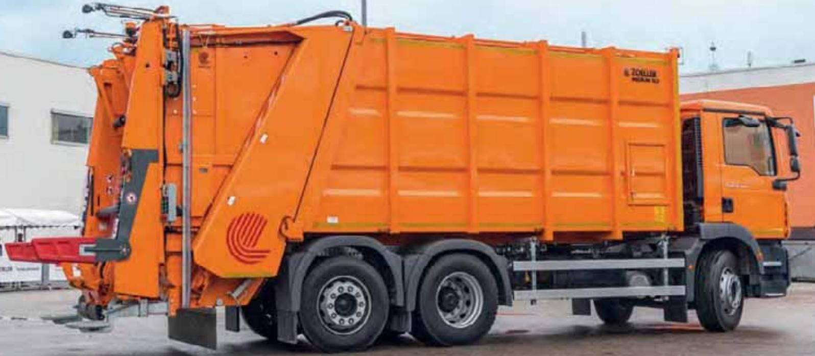
MEDIUM XLS with integrated lifter ZOELLER-ROTARY III, Low-Level with hinged chute
