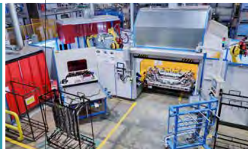
KIRCHHOFF Automotive manufactures the high-voltage clip for the BMW iX1 and Mini Countryman electric on a new welding line at its Iserlohn plant.
