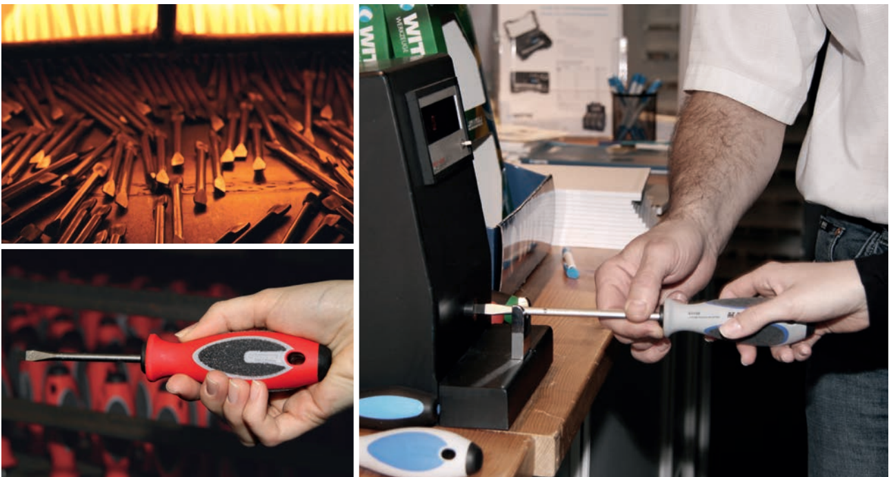
One tempering process step takes place in the oven (top left), which is crucial to the stability of the screwdriver. With the flocked handle of the MAXXPRO (bottom left), good results are guaranteed at the torque measuring station (bottom right).
