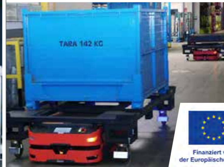
Automated guided vehicles in use at the Iserlohn/Germany plant.
