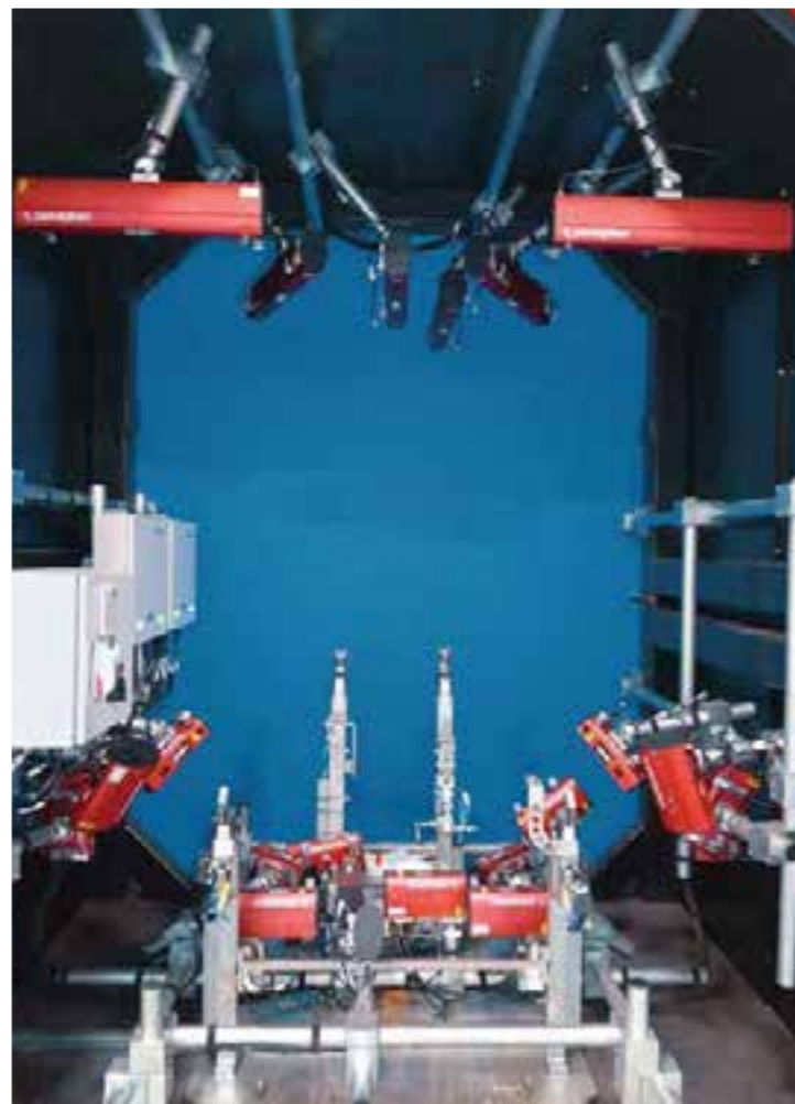
Left/below: Modern technologies are used for quality assurance. For example, weld seams or the geometry of finished products are checked and measured inline.
