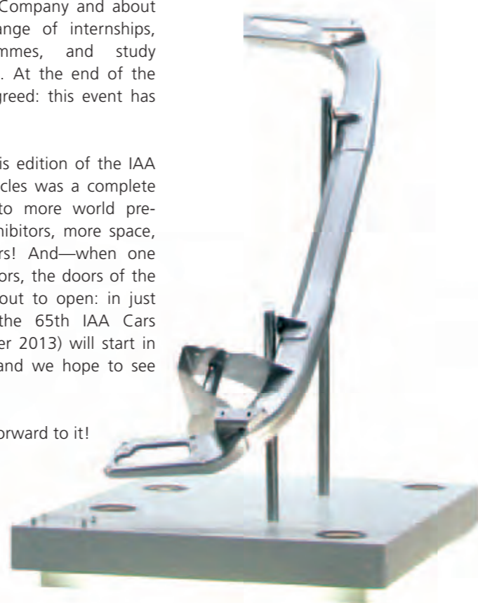
The front underride protection for the MAN TGX and TGS, a product that KIRCHHOFF Automotive is in charge of during all phases of the product life cycle, from design and development through prototyping to series production.
