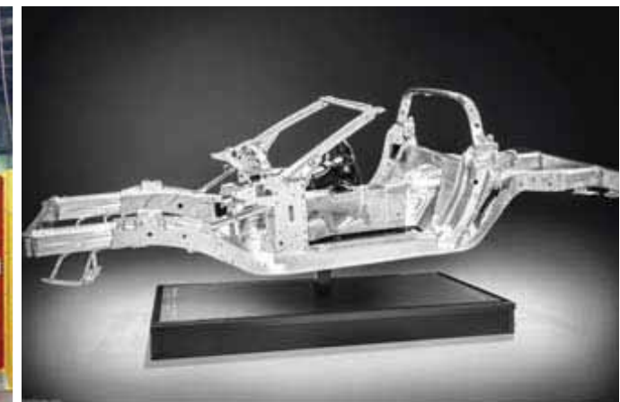
left: Usage of the new General Motors proprietary method for Spot Welding of aluminum | right: C7 Corvette all-aluminum frame
