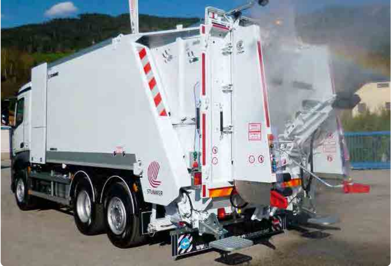
Left: ZOELLER ROTARY automatic lifter and 800 litre steel containers in washing position. In Switzerland the cleaning power of the STUMMER “Waschbär” is also appreciated. The cleaning power can be exceptionally combined in conjunction with the automatic or manual lifting system. Right: The pivoted robotic arms with the wash heads provide perfect cleaning of the waste containers. Around three litres of water are needed per container, with a water pressure of 120 bar.
