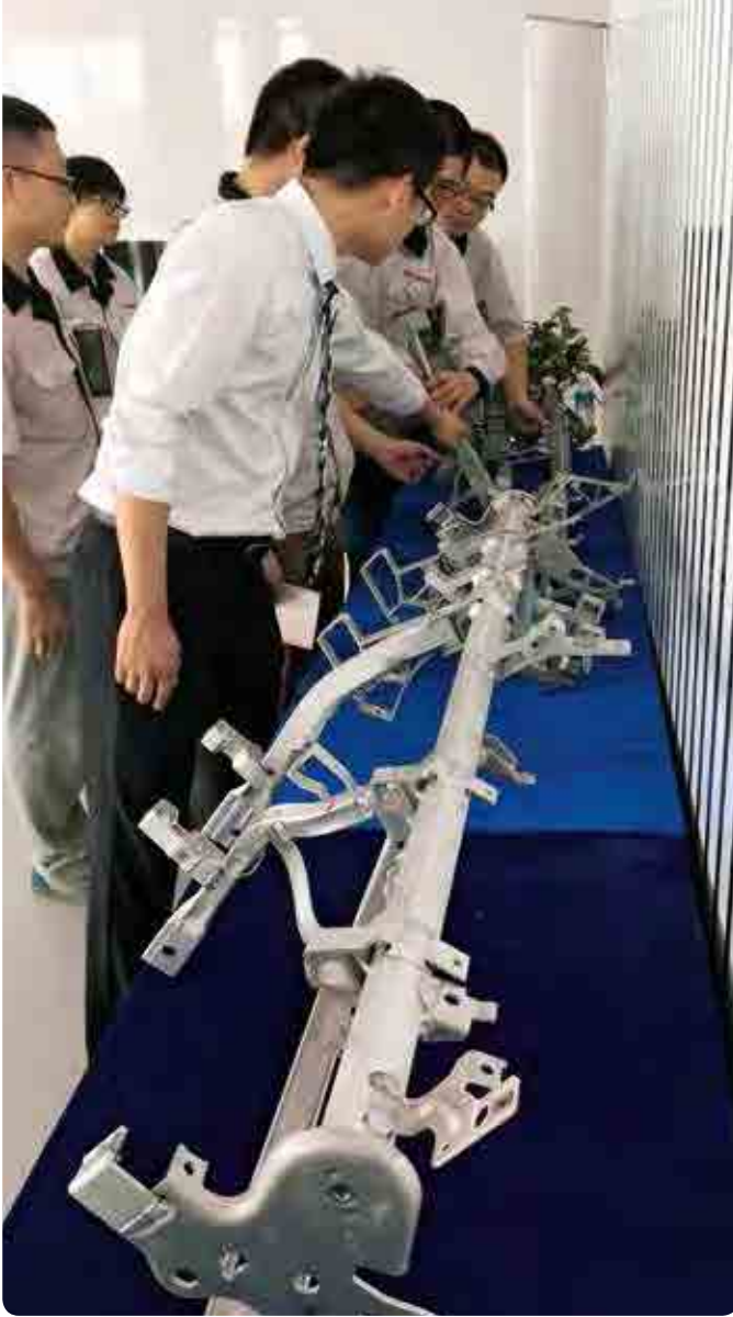
Left: Cross car beams made of aluminum or of laser-welded steel arose great interest among the visitors of Great Wall. Bottom: Wang Guangdong (center), Technology Director of the Automotive Material Engineering Research Institute and the Department of Material Application examines the aluminum products from KIRCHHOFF Automotive.
