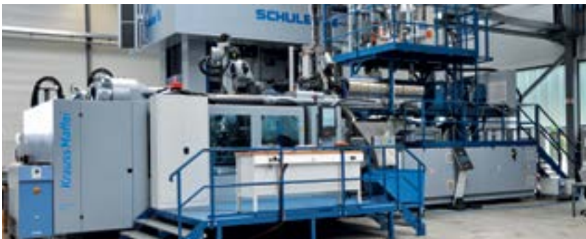
Injection molding compounder with a clamping force of 13,000 kN
